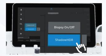
2 Adjust a strength by tapping the [ShadowHDR] button on the flexible menu. (1 - 5)
