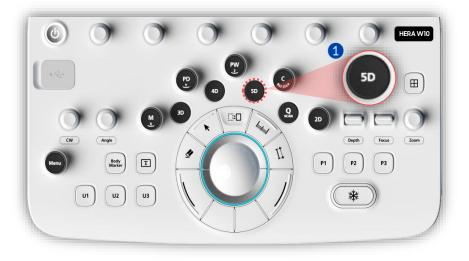
1 5D Button Press 5D button on the control panel.
