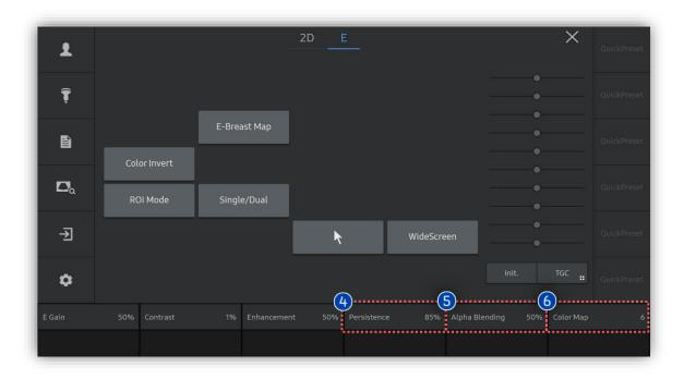
The feature controls the E-Strain frame average. The higher this value is, the higher the frame averaging will be. Increasing the persistence level will reduce the frame rate. For a higher frame rate, decrease the persistence level.
