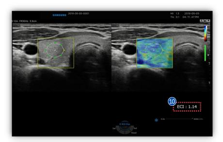
After pressing the [Set] button, ECI (Elasticity Contrast Index) will be calculated and the results will be displayed at the bottom of the display monitor.
