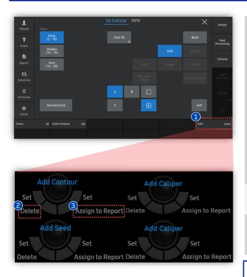
A measurement target will be added based on the seed position entered by the user. You can use this when you find a follicle that has not previously been detected. A measurement target will be added based on the Contour / Seed / Caliper / Ellipse entered by the user.
